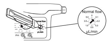
The normal flow can be adjusted in eight different flow rates by the switch at the back of the pump.
